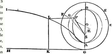
time by its point A describing the cycloid ALI. Which done, take GK to the perimeter GEFG of the wheel, in the ratio of the time in which the body proceeding from A described the arc AP, to the time of a whole revolution in the ellipsis. Erect the perpendicular KL meeting the cycloid in L; then LP drawn parallel to KG will meet the ellipsis in P, the required place of the body.
