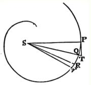
Let that spiral be PQR. From the velocity, with which the body goes over the very small arc PQ, the time will be given; and from the altitude TQ, which is as the centripetal force, and the square of the time, that force will be given. Then from the difference RSr of the areas PSQ and QSR described in equal particles of time, the retardation of the body will be given; and from the retardation will be found the resisting force and density of the medium.
