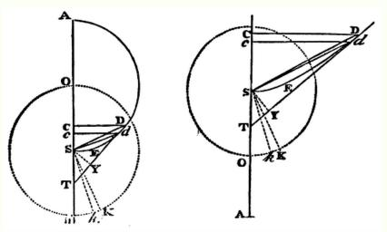
For suppose a body C in the smallest moment of time describes in falling the infinitely little line Cc, while another body K, uniformly revolving about the centre S in the circle OKk, describes the arc Kk. Erect the perpendiculars CD, *cd*, meeting the figure DES in D, *d*. Join SD, Sd, SK, Sk, and draw Dd meeting the axis AS in T, and thereon let fall the perpendicular SY.
